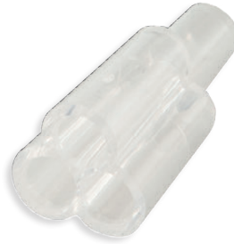
Clear, 3-Way Connector Tubing Pockets Connector 1: .160" Tubing Pocket Connector 2: .160" Tubing Pocket Connector 3: .160" Tubing Pocket Material: Cyrolite
